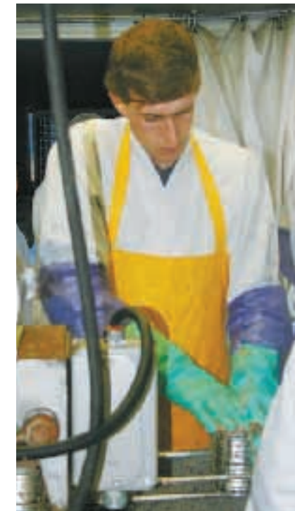
5. The cooked meat is packed firmly into cans and sealed. The cans are then cooked for a further two hours in a retort steam cooker.
