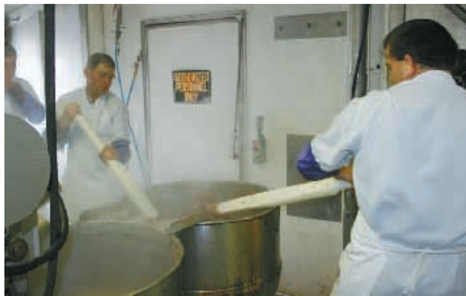
4. The cubes of ground beef are cooked—300 pounds at a time—with salt in large steam kettles. Keeping the meat from sticking, and to ensure even cooking, requires constant stirring.
