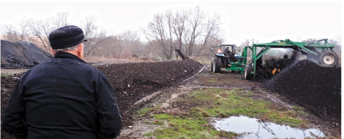
Edwin Sittler, an Old Order Mennonite, watches as a machine he designed turns a windrow of compost.
